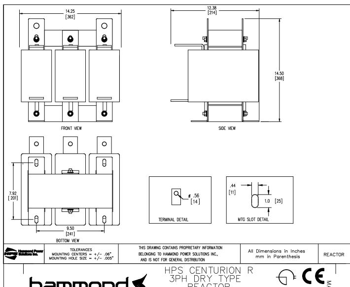
HPS CENTURION R 3PH DRY TYPE REACTOR
