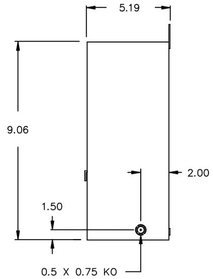
FRONT & BOTTOM PANEL IS HINGED FOR ACCESS TO TERMINALS, BOTTOM MOUNTING HOLES AND REAR KNOCKOUT.
